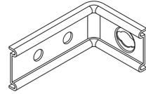
CANTONEIRA METALICA PARA FIXAÇÃO NA PAREDE       | <b>4</b>   | <b>J</b>
